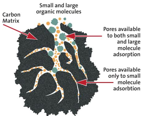
Contains a maze of tiny pores with sizes ranging from 500-1000 nm and a surface area of about 1000 square meters per gram. The nature of this surface allows adsorption of organic impurities from the water and catalytic decomposition of free chlorine and, more slowly, chloramines.
